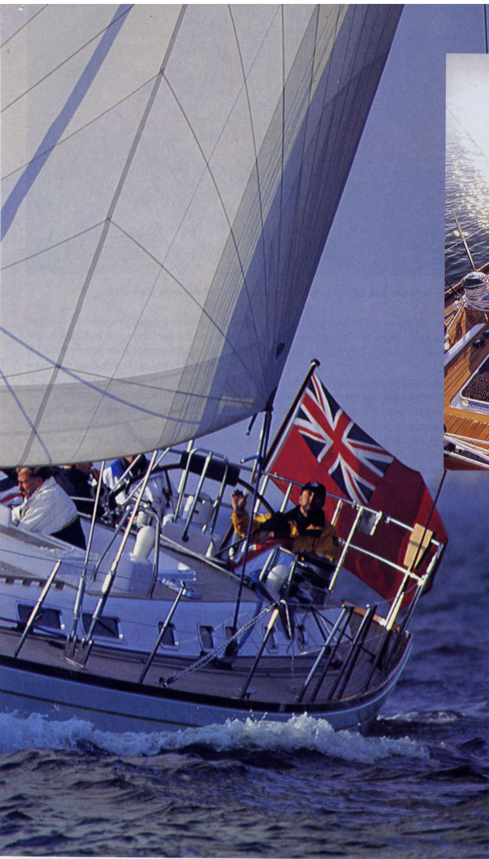
Above , all controls are led back to the after steering cockpit, equipped with a Lewmar winch package. Below , Song of Nike's rig is slightly taller than the standard option
