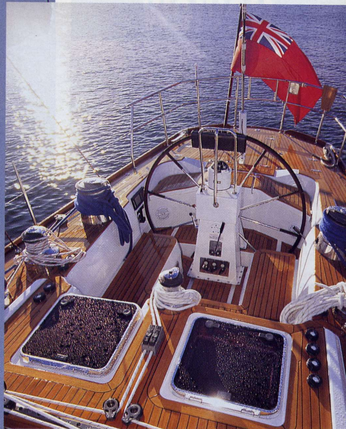
Above , all controls are led back to the after steering cockpit, equipped with a Lewmar winch package. Below , Song of Nike's rig is slightly taller than the standard option
